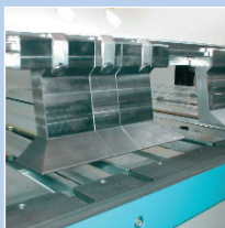
Segmented snap-in box and pan tooling.
